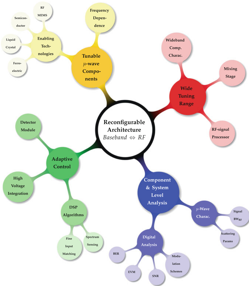
Fig. 1.2 Overview of study areas for the realization of a reconfigurable transceiver architecture towards multiband and multistandard functionality proposed in this work
